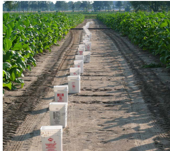
Figure 10 Irrigation assessment catch buckets (Photo courtesy of Rebecca Shortt, OMAFRA)
