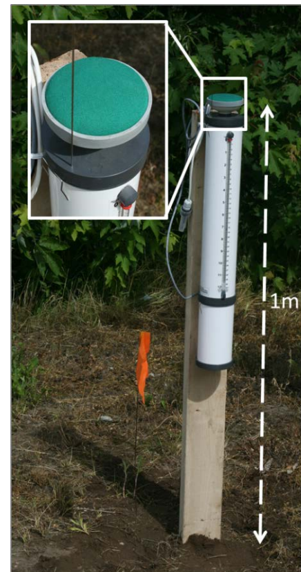
Figure 5 Evapotranspiration gauge set up at the Burford Tree Nursery.
