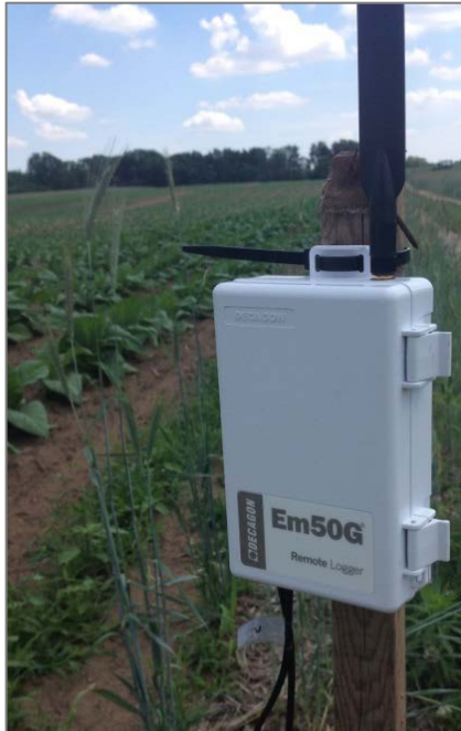
Figure 4 Decagon Em50G Remote Sensor on a tobacco field.
