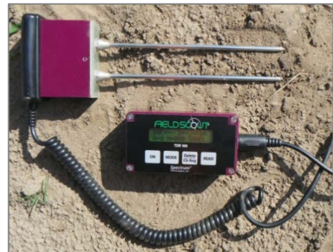
Figure 3 FieldScout TDR100 Soil Moisture Meter with 8" probes.
