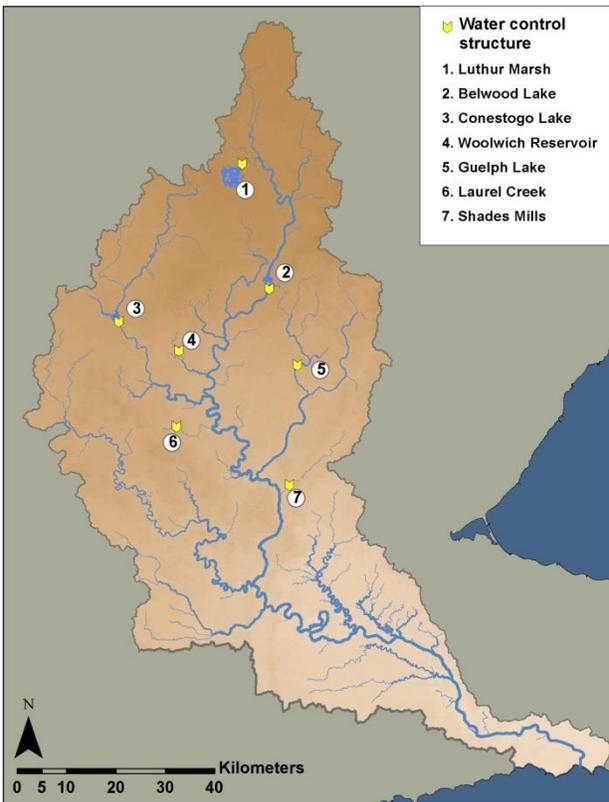
**Figure 4. Location of the water control structures that provide flood control and low flow augmentation**
